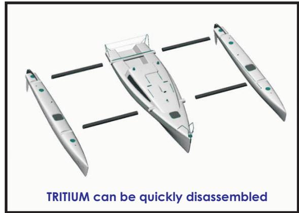
TRITIUM can be quickly disassembled
